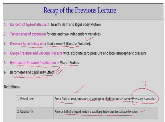
In the last class just to have these things that we derived the pressure force acting on the fluid and or the control volume. And also we know it how the pressure, the hydrostatic pressure distributions it just varies along the z direction when you simplify the problems and on a horizontal surface, the pressure becomes constant. So those the hypothesis we will use it now for derive the equations for manometer or the inclined submerged surfaces.
