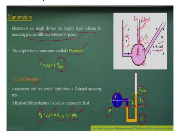
Now let us come to the manometer. Very simple devices are used to measure the pressure like you have a, let have these type of conduit, the pipes the carrying any liquids and you want to measure it what could be the pressure on that pipe. So we can just insert the tubes like you can see can have the tube like this or can have a tube like this with inclined and all or you can have a inclined like this.
