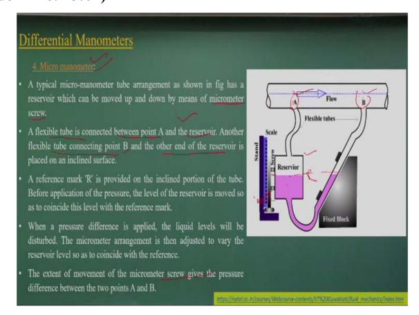
Now there are a simplified micro manometers are there which is a measure the pressure difference between A and B and you have the flow. This flow may be carrying oil or maybe carrying slurry. It maybe carrying any industrial if you look it the any industry is a lot of pipe networks and we have to measure the pressure difference between two points, which is required to measure the discharge, to measure the frictional losses and all.
