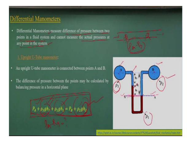
Mostly we are looking it at the two points like I have the pipe and I have the point A and B. So this is a pipe flow, I have the point A and B. At this A and B locations, I want to know it what is the pressure difference between these two point of A and B in this pipe flow. I am not worried about the absolute pressure at the A or the absolute pressure B.
