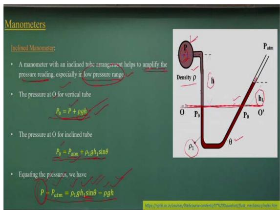
Another case let we have an inclined manometer which is have a quite advantage in the sense that it amplifies the pressure reading as compared when you talking about low pressure ranges. When you are measuring the low pressure ranges it being inclined so it is a give a easier for us to measure the low pressure as compared to the vertical one.
