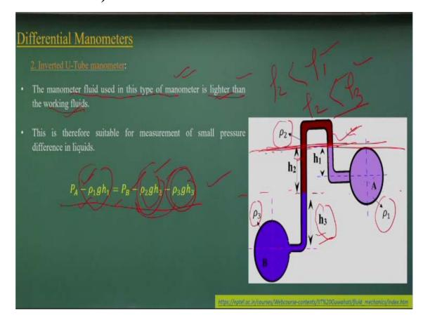
Now if you look it if I have a inverted U tube okay that is inverted cases okay, this is the meter. When you use the manometer fluid use in this type of manometer is lighter than the working fluids. So these are two are the working fluid, which is having this  $\rho_1$  and  $\rho_3$  at two different density of the working fluid. But  $\rho_2$  is the density of the manometric fluid.
